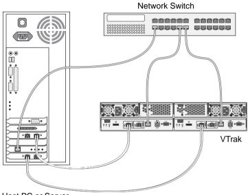
Figure 12. VTrak E310f DAS data and management connections
